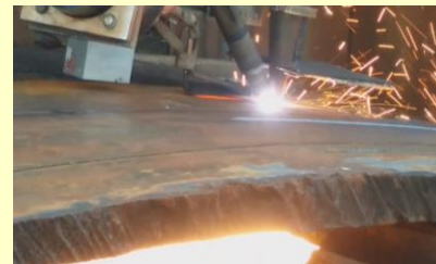
Hybrid Induction thick steel cutting. Portable system for cutting thick steel plates at 7X faster than automated plasma or oxyfuel cutting
