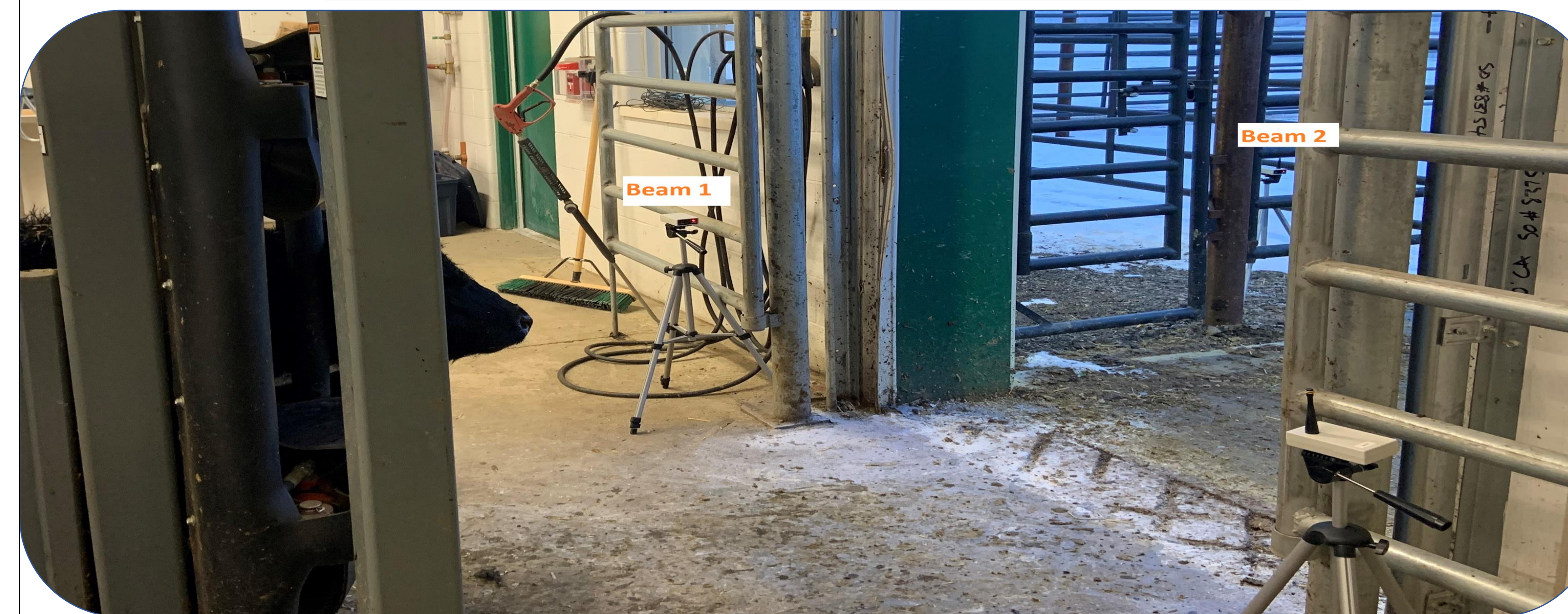
Fig. 2: Flight speed device used to measure cattle temperament.
