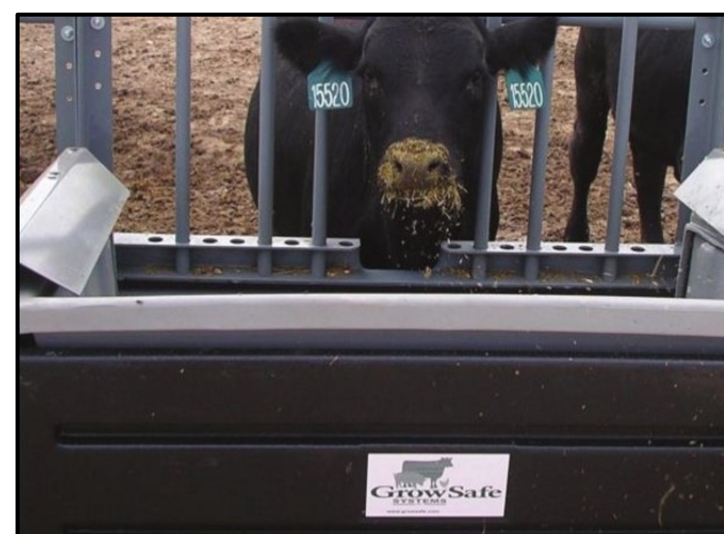
Figure 2. The GrowSafe Feed Intake System is equipped with a scale and electronic identification tag reader that collects data on individual animals.
